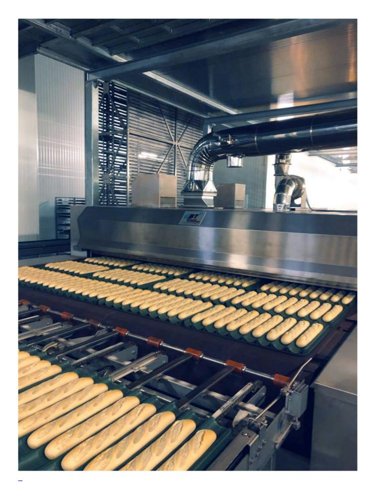
This industrial bread baking plant situated near Barcelona reaches an output of up to 5,000 pc. par-baked baguettes thanks to GBT's oven Mistral. Far beyond: The energy optimized modular conveyor oven saves up to 30% of energy in comparison with a conventional cyclothermic oven. This is possible due to the specially developed use of the flue gases energy. Typically GBT: maximizing output, reducing energy consumption.
