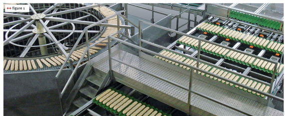
++ Figure 1 The spiral conveyor for cooling
