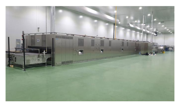
The new GBT oven Mistral convinces with even heat from the first baking. The baking behaviour is similar to a thermal oil oven. With a 50% lower power input than a conventional cyclothermic oven, with the use of conventional household burners for gas or oil use and the cleverer modular design allows flue gas utilization, which can end up saving up to 30% energy. Very short installation time, no welding in bakery.
